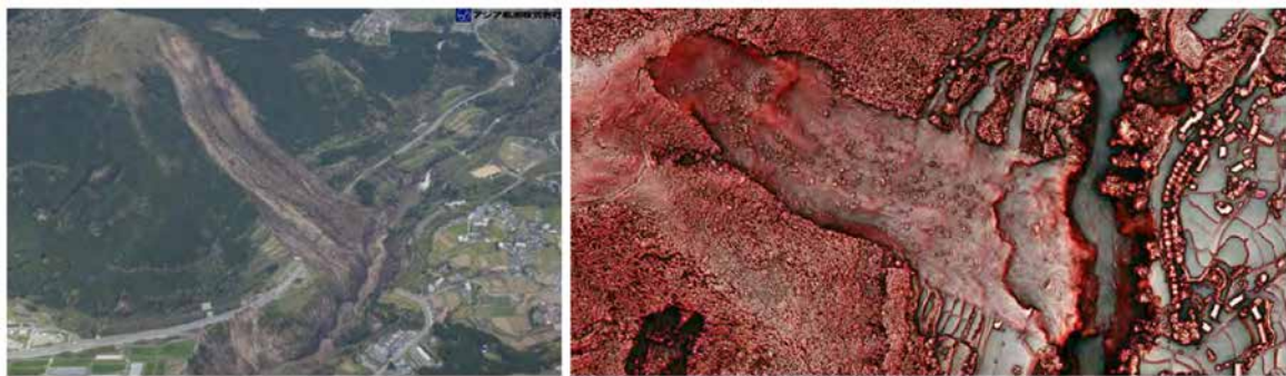
Figure 2-4: The Aso landslide was triggered by the Kumamoto Earthquake, April 16, 2016. Left: Aerial photograph was taken after a few hours later the earthquake occurred; Right: RRIM of the Aso landslide using Airborne Lidar data taken on April 16.
